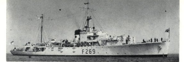
The last 'River' class to be actively employed in the Royal Navy was HMS Meon. Notice the revised gun armament, exclusively of close-range weapons, and particularly the special Oerlikon sponson above the post-war pendant number. As an HQ ship for landing craft, she had an extensive radio system, and wore the 'Combined Ops' badge on her funnel beneath the 'leaders' band.
